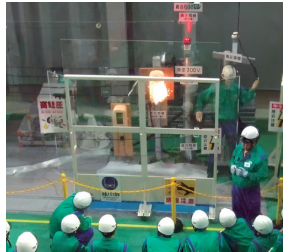
Reproduction of a short circuit
