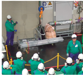
Reproduction of a suspended load fall
