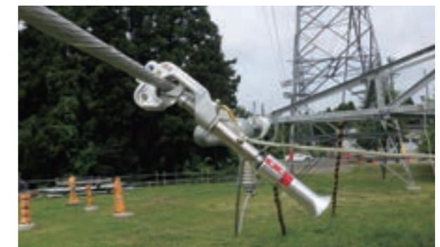
● Major industrial property rights: Patent No. 7390460 "Short-circuit grounding instrument and grounding construction method using the same"
