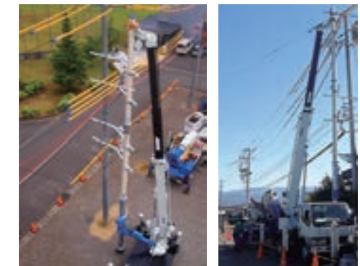
● Major industrial property rights: Patent No. 6499789 "Device for utility pole replacement using the original hole, vehicle for utility pole replacement using the original hole, and utility pole replacement method using the original hole"
